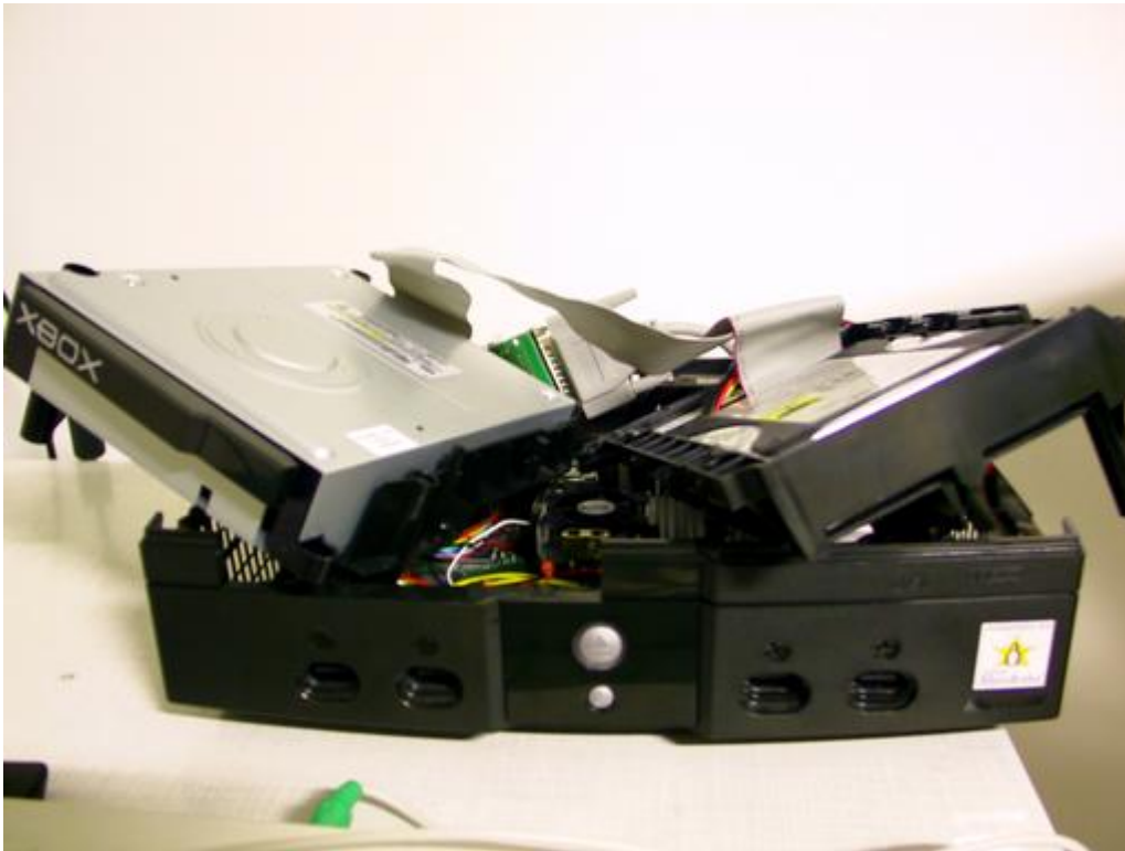
Figure 3. The Xbox dissected: the Philips DVD drive is on the left, and the Seagate hard disk is on the right. The green board in the background is a modchip that is, in this case, connected to a computer's parallel port.
