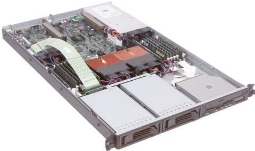
Figure 1. The Newisys 2100 puts two Opteron processors in a 1U enclosure.
