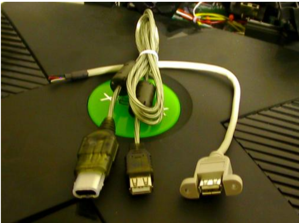
Figure 4. A USB adaptor cable can be built easily by using an XBox controller extension cable and the USB female connector on the right. You also can buy prebuilt cables like the one on the left.
