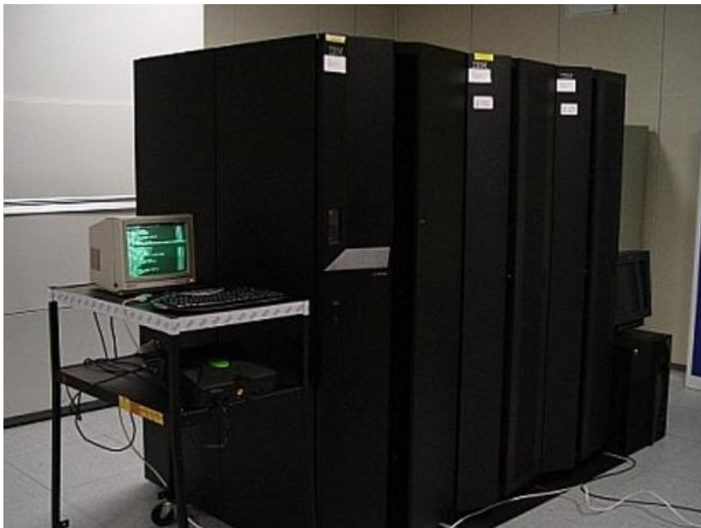
Figure 5. A German data center is using an Xbox-based Domino Server, running a clustered environment with Domino on an IBM pSeries. The Xbox is the small system on the left.
